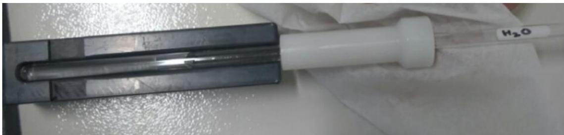
Figure 1. NMR tube inside the block. Measure the correct depth by slightly against the block. Don't touch the Teflon holder using bare hands. Always use Kim wipe.
