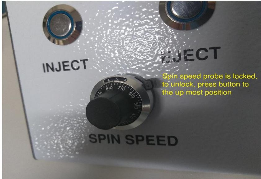
Figure 7. The control box has a knob to control the spin speed.
