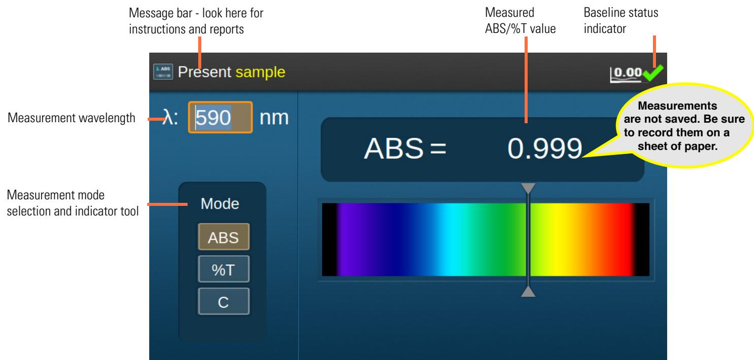
Live Display shows a continuously updating value for the transmittance, absorbance or concentration of a sample. The instrument takes a new measurement every two (2) seconds. The value on the screen flashes to indicate that a new reading is being displayed.
