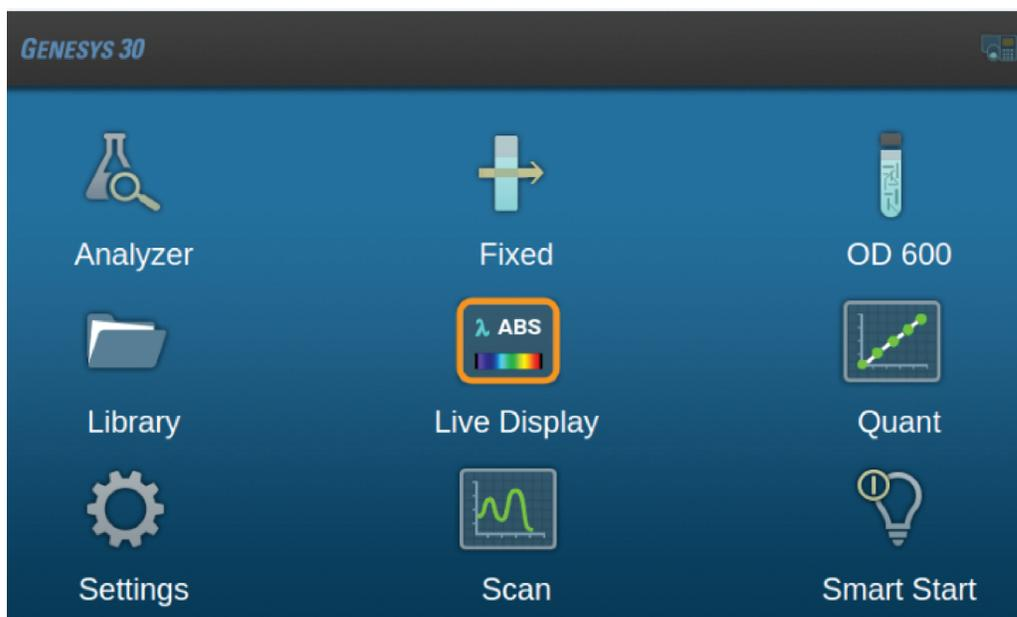
Options are clearly labeled with the name of the measurement modes or functions that they execute. Use the nav keys to select the desired application and press
