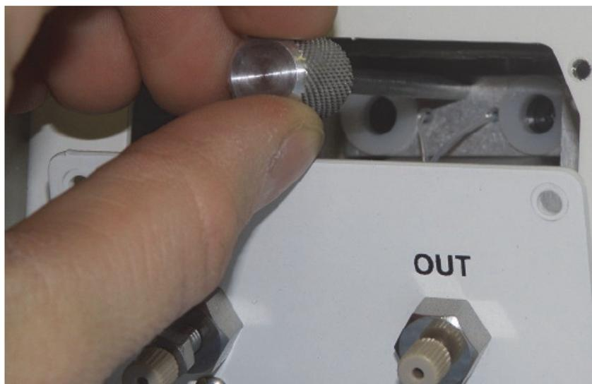
There are two bolts that secure the cartridge flange to the magnet. They can be loosened with the long-handled hex wrench supplied with the replacement cartridge. The bolts are located behind white plastic bushings, as shown in [Figure 3](#). The bushings will retain the bolts so that they cannot fall out and become lost inside the unit. Loosen the bolts alternately until they disengage from the threads.
